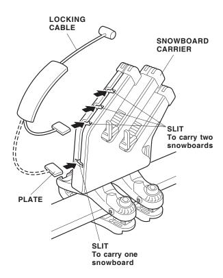
15. After loading the snowboards on the carrier, adjust them with the help of the board supports so that the top edges are level and the boards are as far down in the carrier as possible. To secure the snowboards, use the key to open the covers, then insert the locking cable barrels into the holes in the carrier covers.
